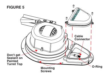
**STEP 5:** Make cable connections from wires on the roof, to wires in mount. Apply approved sealant around cable entry hole. Replace cover over cable area making sure O-Ring is in place. Then tighten the three cover screws. See Figure 5.
